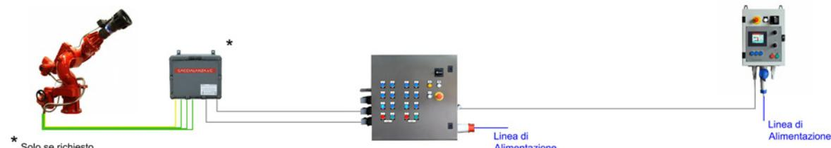
In any case the power panel is equipped with a special socket for direct connection of a portable command unit by means of a mobile cable whose max. length is 30 m.
