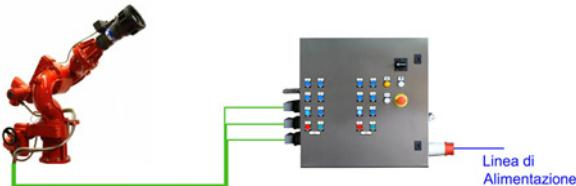
For longer distances between the panel and the monitor a terminal cabinet has to be installed near the monitor.
