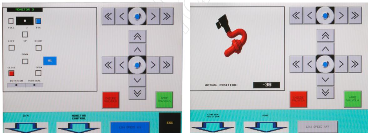
For each monitor all the operations can be performed both from the power and command panel associated to the monitor involved and from any fixed or portable command panel.
