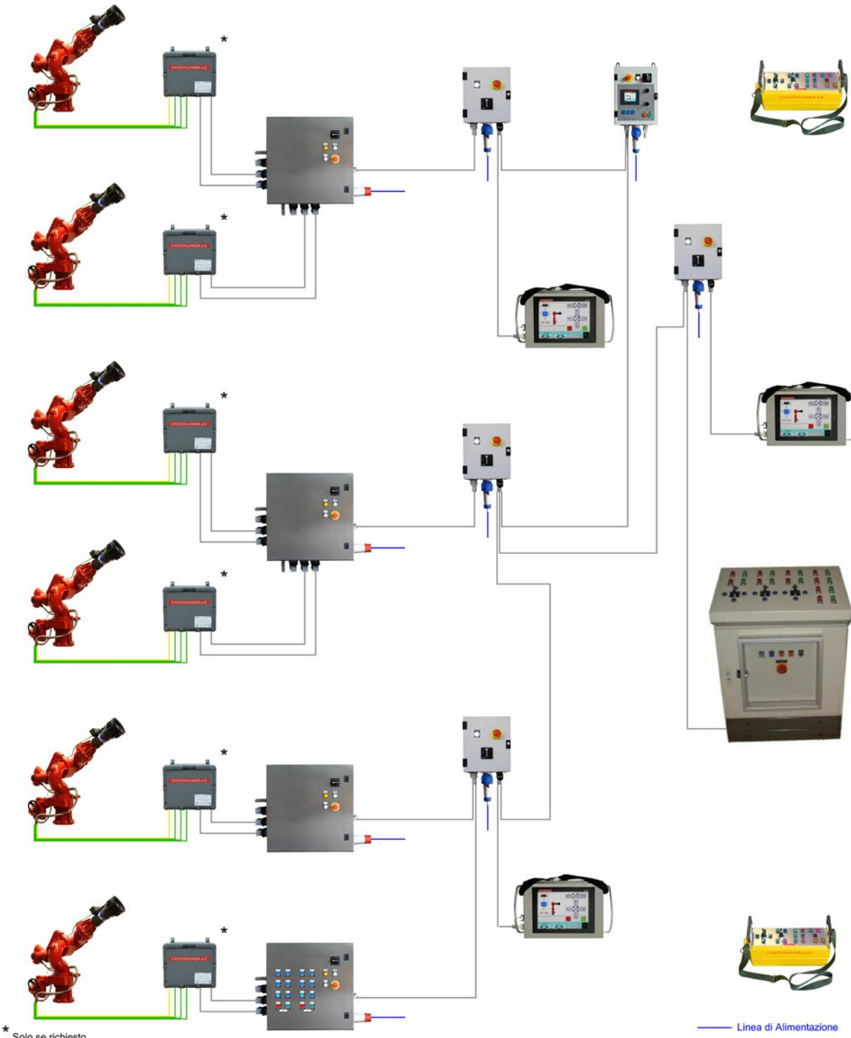
All the above can be supplied also in deflagration proof execution for installation in hazardous areas (explosion danger). In such a case monitors and power panels are supplied in ATEX Eexd execution.
