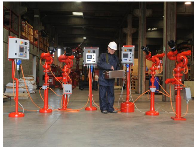
A monitor system consists of the required number of monitors, their standing poles (if the monitors are required in elevated position) and the command and control panels.
