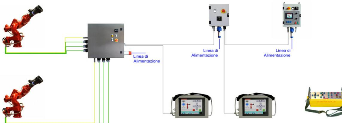
The portable panels with radio connection have all the functions available for the other command panels.
