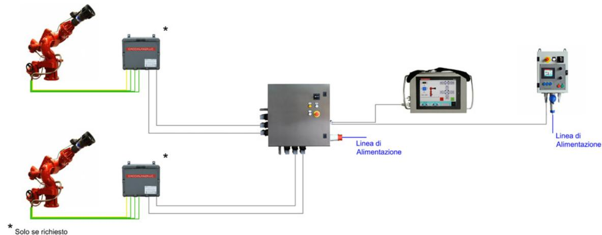
An additional remote command panel can be connected to the power and command panel. The connection between the two panels is performed by means of a single cable according to communication standard modbus or ethernet.
