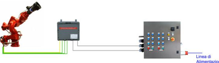
Monitor commands can be placed in a control panel separate from the power panel. The power panel can be equipped also with local commands, or not, as required. In the same way there can be or not the terminal cabinet between the monitor and the power panel according to the requirements.
